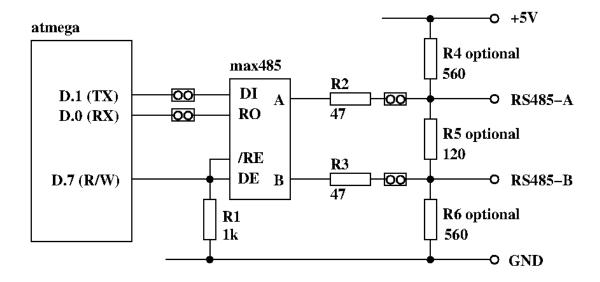
An RS232 - RS485 converter of some sort is needed to connect the serial interface of the collector computer to the bus. USB - RS485 dongles are available as well. Please note, that the connector should not produce a local echo of the bytes transmitted, or software needs to take care of the double echo. The controllers are sending an echo character as well, this serves as handshake when uploading forth code, too.
